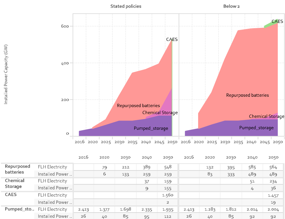
Figure 11-27 Storage capacity (GW) and full load hour development in the two scenarios.
