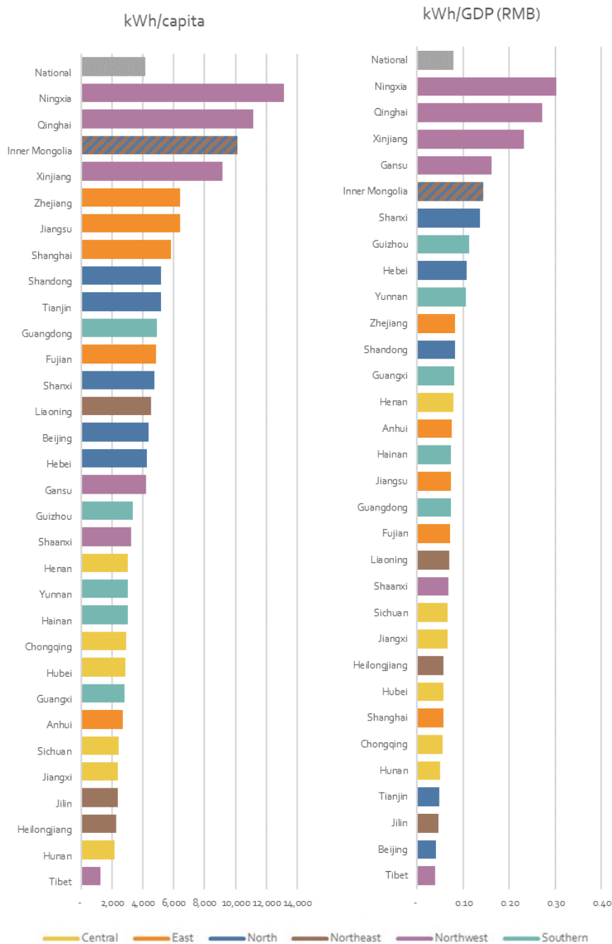
Figure 11-7 2015 electricity consumption per capita (l) and electricity consumption per GDP (r) Source: Calculations based on National Bureau of Statistics
